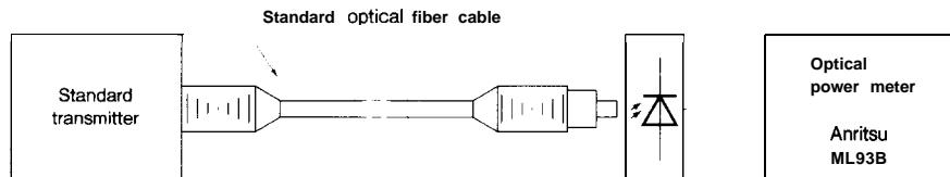
Standard light transmitter : Light transmitter that provides the fiber-end optical output of  $-15\text{dBm} \pm 0.3\text{dBm}$  when the standard optical fiber cable is connected.
