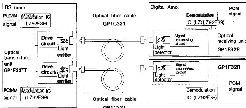
\*LZ92F39 is Sharp's modulation/demodulation IC
