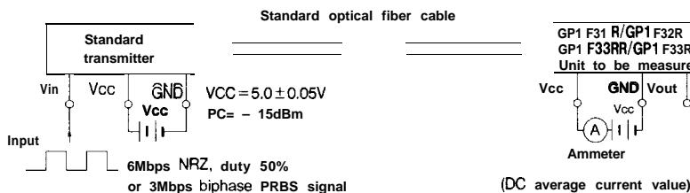
\*13 output voltage/Pulse response measuring method
